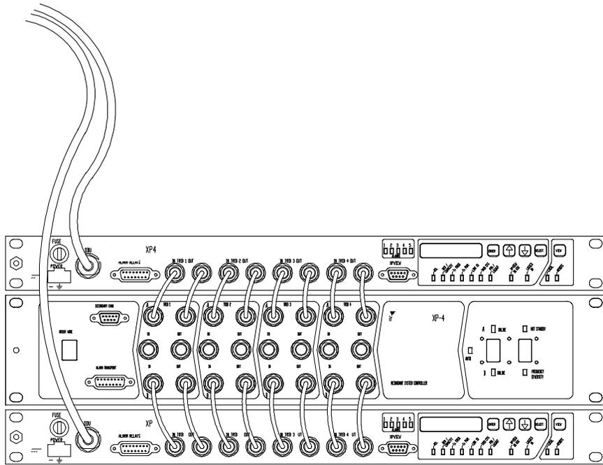
Figure 2-3. Unbalanced 2x/4x IDUs in Protected Configuration.
