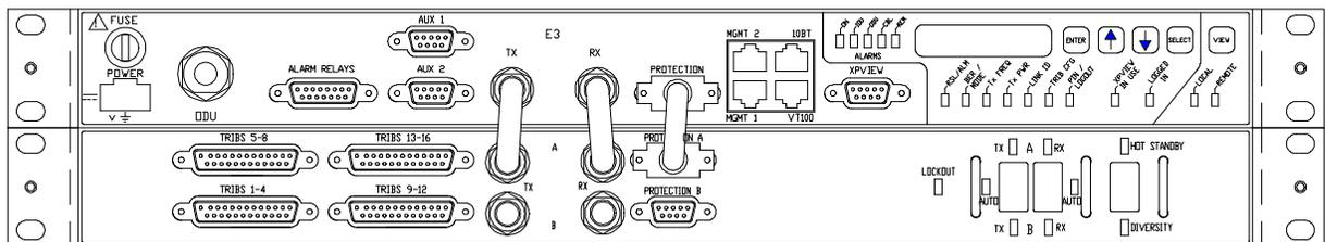
Figure 4-4. 16E1 IDU/MSU Front Panel Connections
