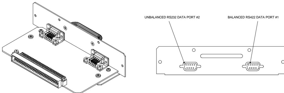
Figure 7-21. IDU Auxiliary Data Channel Option Card for 2x/4x Configuration
