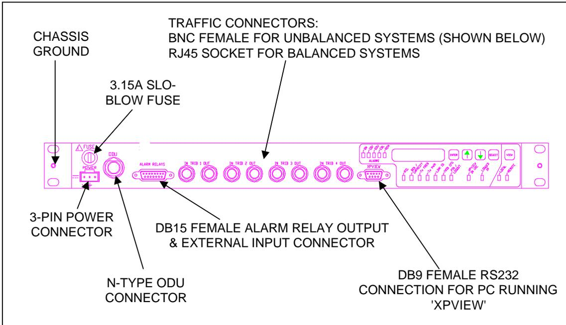
Figure 4-1. 2x/4x IDU Front Panel Connections
