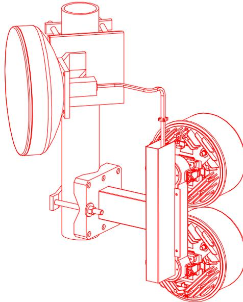
Figure 7-9. ODU Protection Configuration using a Single Antenna
