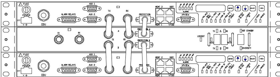
Figure 2.6. Unbalanced E3 or DS3 IDU Protected Configuration
