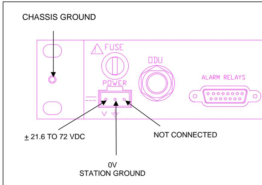
Figure 4-5. IDU Power Connector Detail
