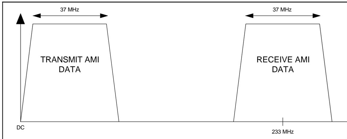
Figure 1-17a. XP4 E3 Cable Signals
