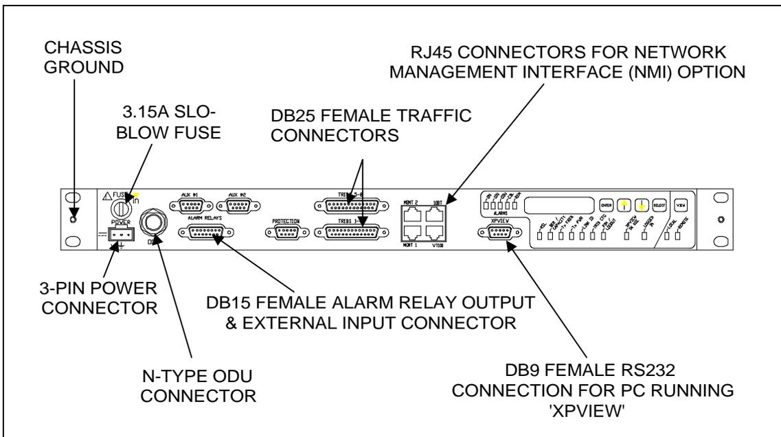
Figure 4-2. 4x/8x and Front Access 2x/4x IDU Front Panel Connections
