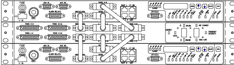
Figure 2-5. Balanced/Unbalanced 4x/8x IDUs in Protected Configuration.
