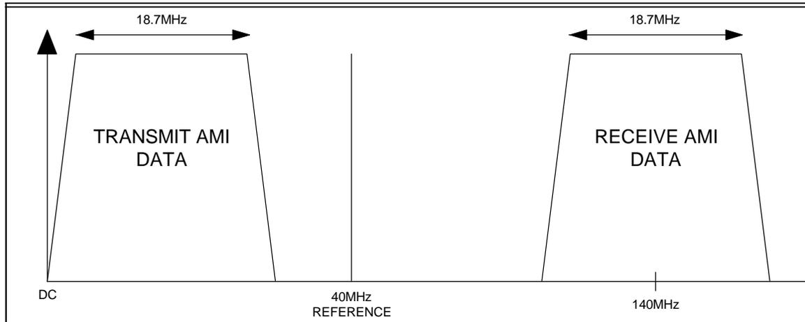
Figure 1-16. XP4 2x/4x/8x Cable Signals
