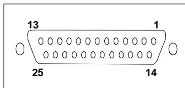
Figure 7-17. VT100 Interface DB-25 Female Connector
