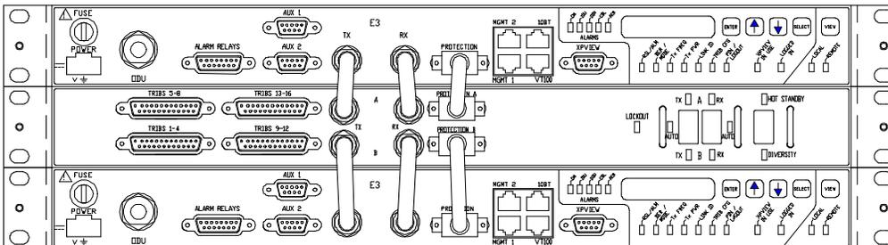
Figure 2.7. Unbalanced/Balanced 16E1 Protected Configuration
