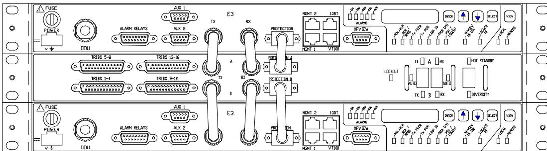
Figure 7-11b. Cable Connections for 16E1 Protected System
