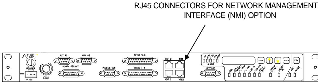
Figure 7-15. SNMP Connection for 4x/8x IDUs
