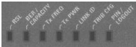
These LEDs indicate the type of data displayed on the 7x7 display.
