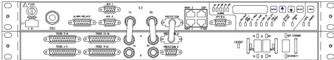
Figure 1-13. Unbalanced/Balanced 16xE1 IDU with MSU
