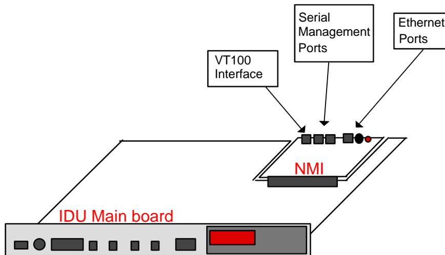
Figure 7-14. SNMP Connection for 2x/4x IDUs
