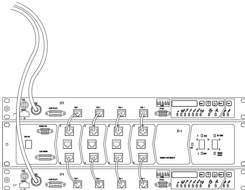
Figure 2-4. Balanced 2x/4x IDUs in Protected Configuration.
