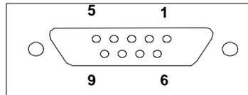
Figure 7-20. RS232 SLIP/PPP DB-9 Female Connector
