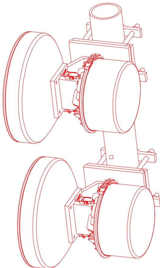
*Figure 2-2. ODU Protection Configuration using Dual Antennas.*
