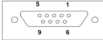
Figure 7-18. VT100 Interface DB-9 Female Connector
