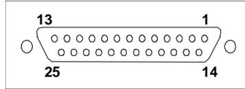
Figure 7-19. RS232 SLIP/PPP DB-25 Female Connector
