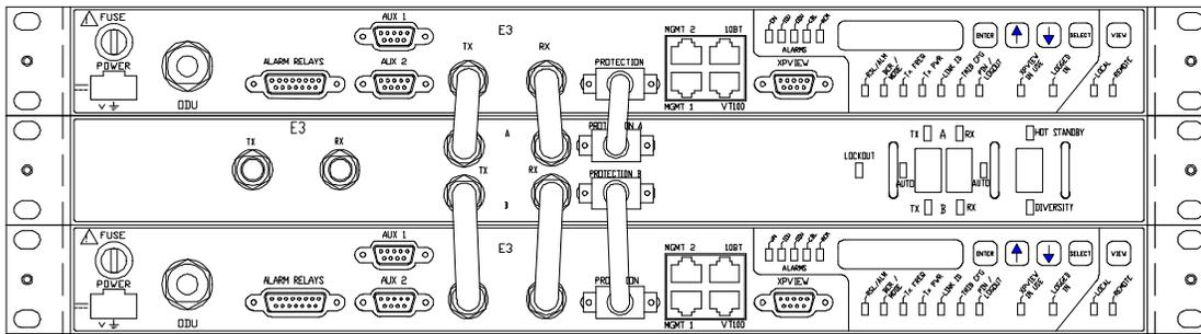
Figure 7-11a. Cable Connections for E3 and DS3 Protected Systems
