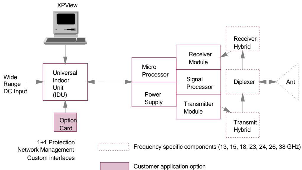
Figure 1-7. XP4 universal radio architecture
