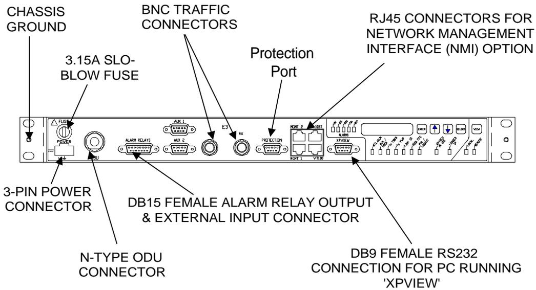
Figure 4-3. E3 and DS3 IDU Front Panel Connections
