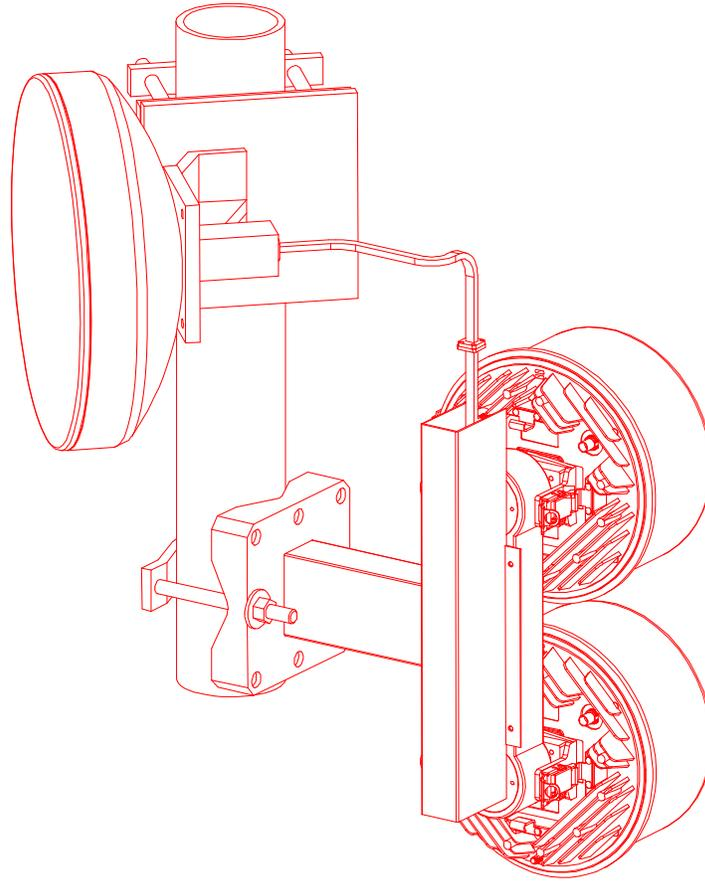
*Figure 2-1. ODU Protection Configuration using a Single Antenna.*
