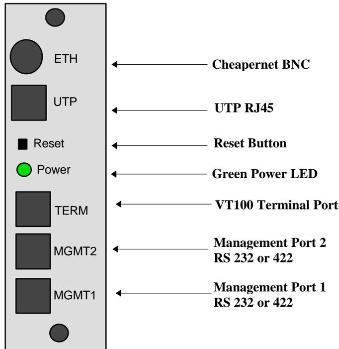
Figure 7-16. SNMP Front Panel for 2x/4x Systems
