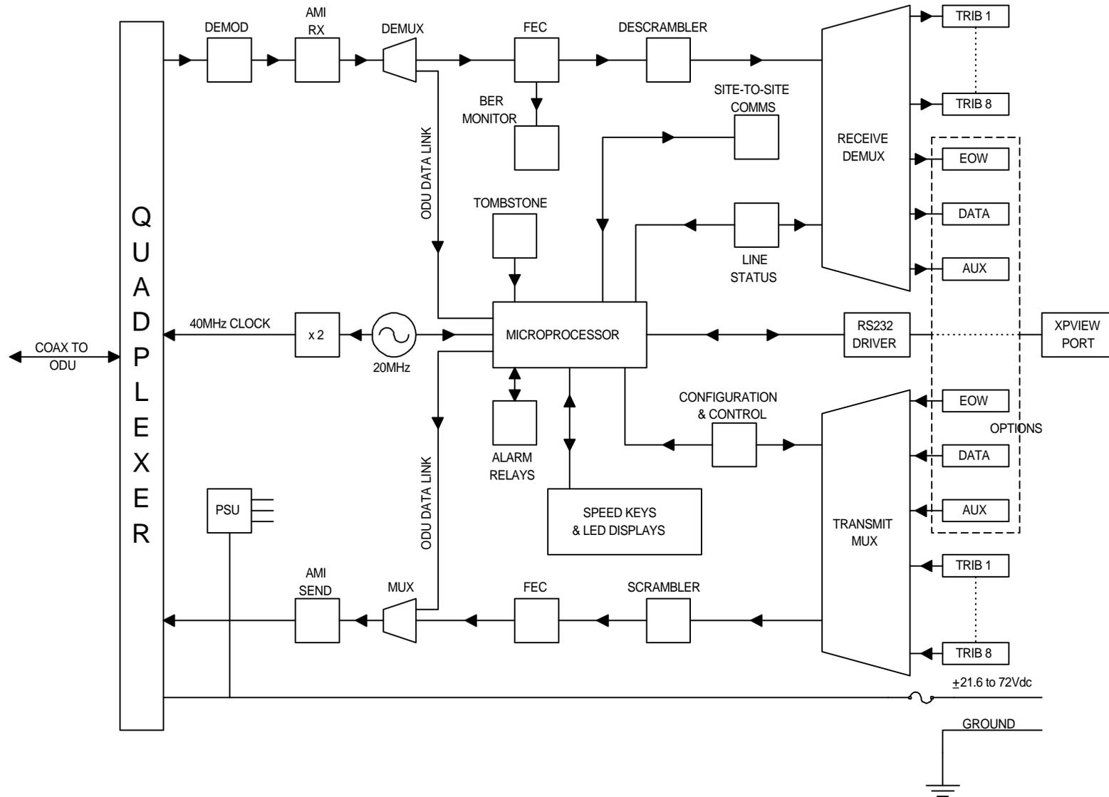
Figure1-14. XP4 IDU Block Diagram
