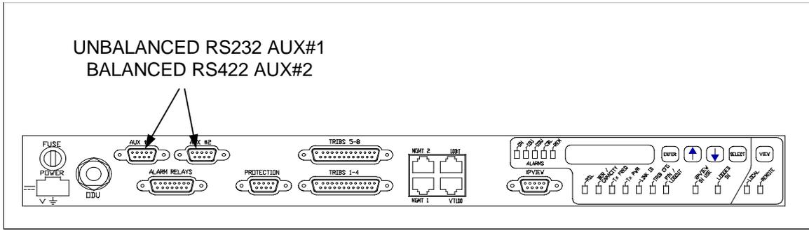
Figure 7-22. IDU Auxiliary Data Channel Connectors on 4x/8x IDU
