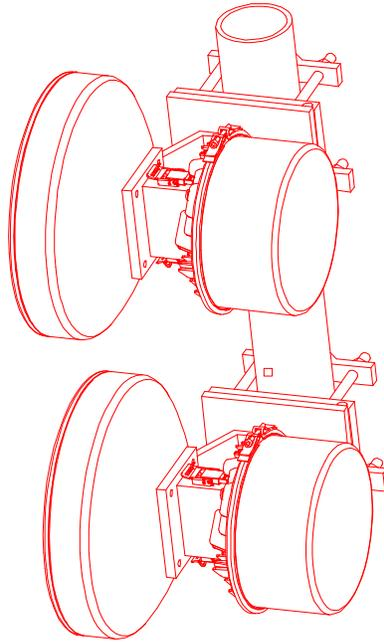
*Figure 7-10. ODU Protection Configuration using Dual Antenna*
