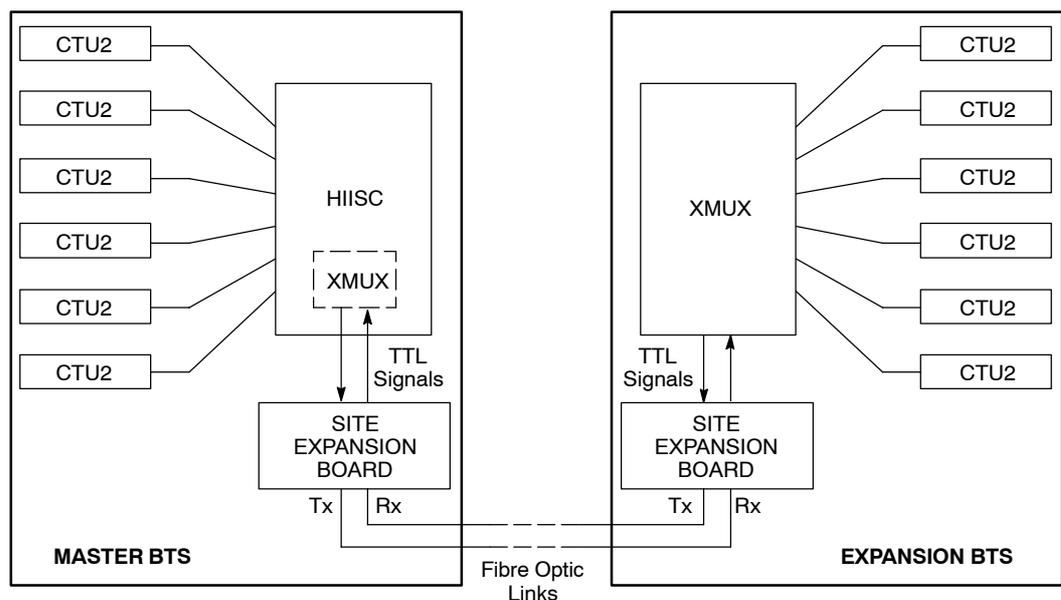
**NOTE** Site expansion is not restricted to using Horizon II *macro* cabinets as slaves. Horizon*macro* and/or M-Cell6 (equipped with a FMUX) can also be used. Similarly, the master BTS can be a Horizon*macro* or FMUX-equipped M-Cell6, with a Horizon II *macro* as one or more slaves. Refer to **Installation & Configuration: Horizon II *macro*** (68P02902W97) for full details of BTS interoperability.
