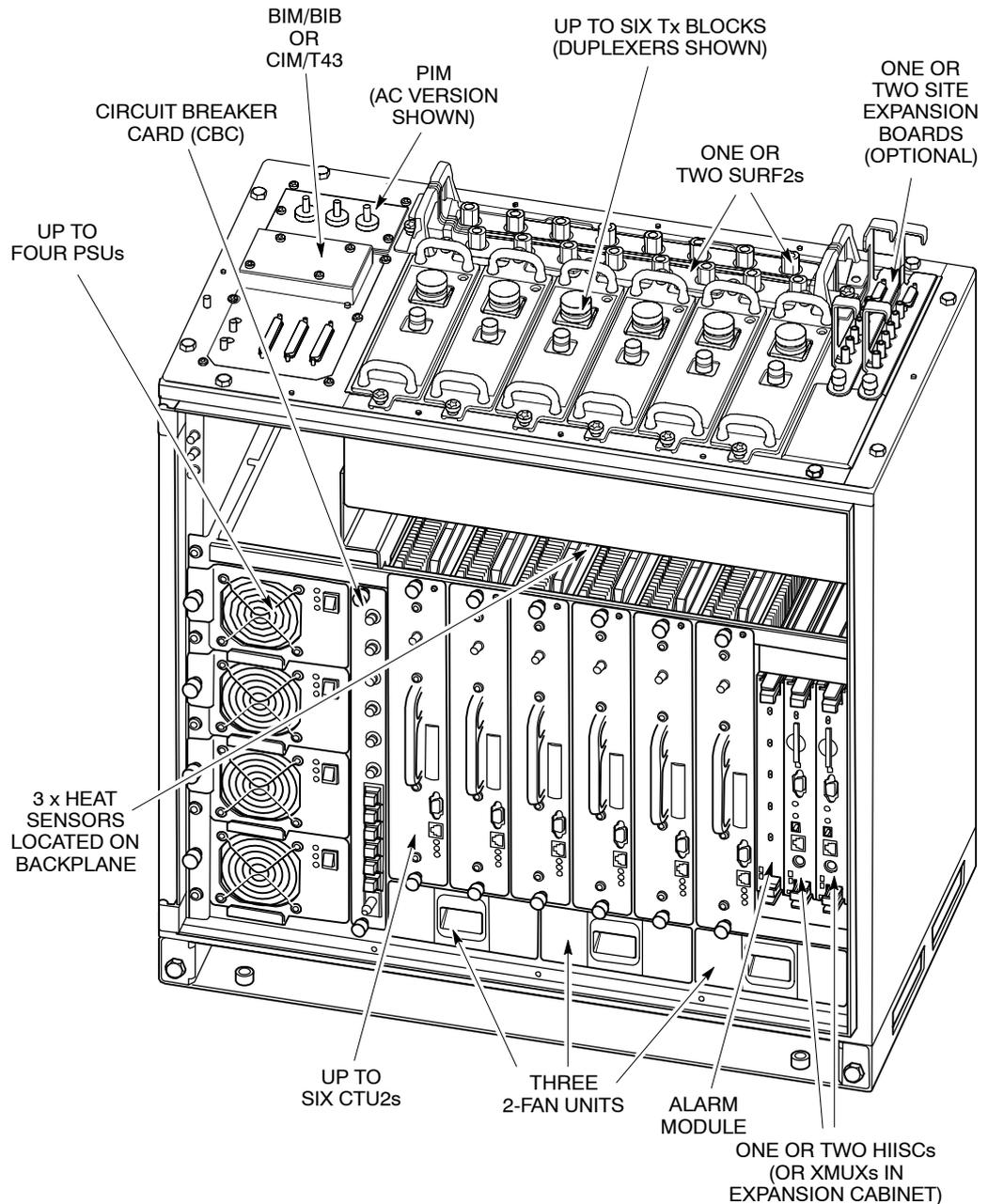
Figure Maint. 4-2 Additional Horizon II *macro* FRU components
