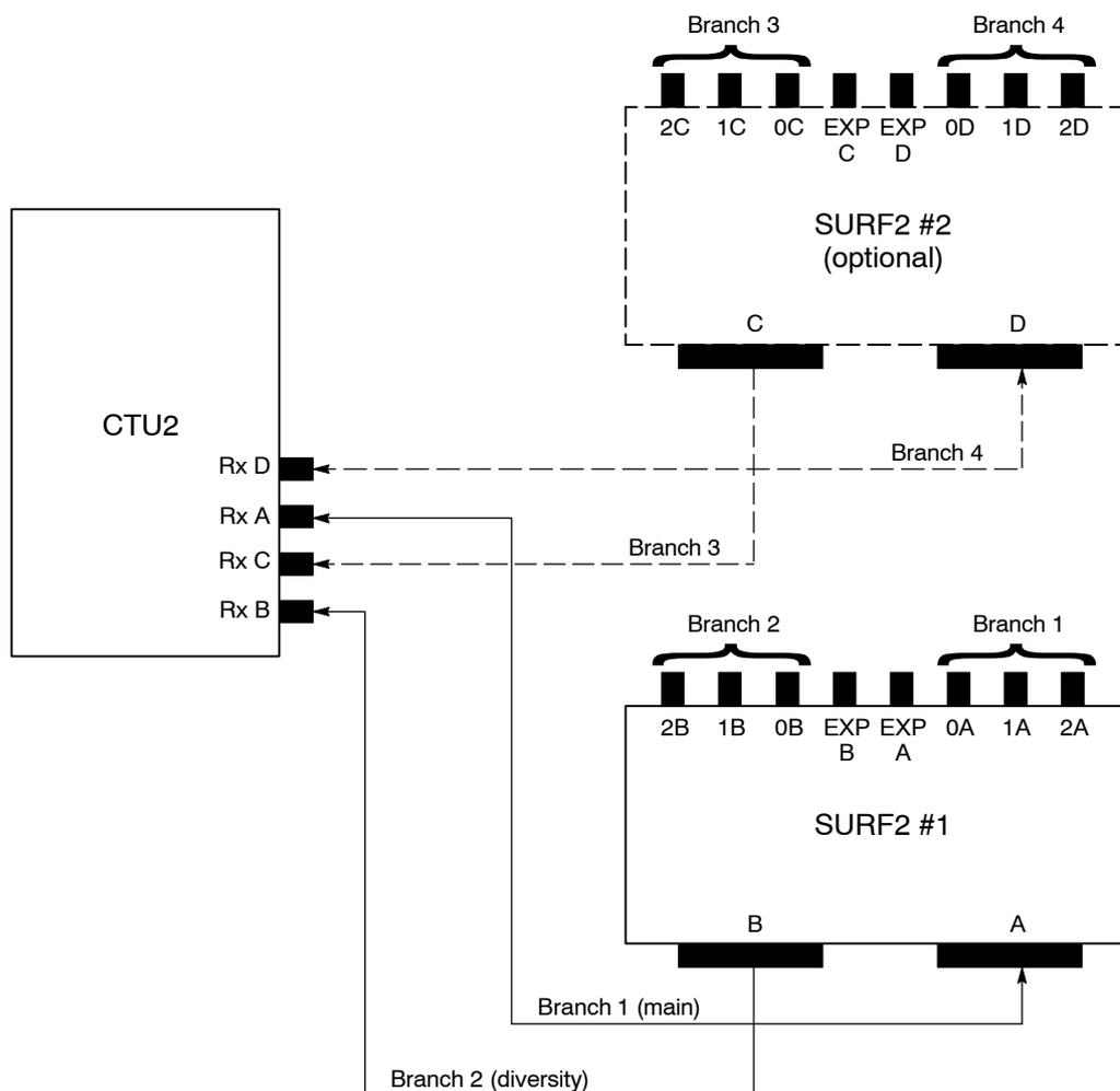
**NOTE** Rx A and Rx C on the CTU2 carry the SURF2 control and alarm signals.
