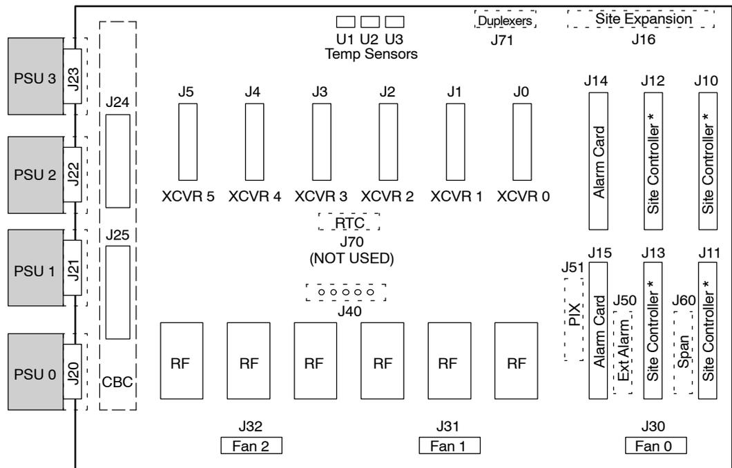
\* The site controller (HIISC) may be replaced by an XMUX in expansion cabinets.
