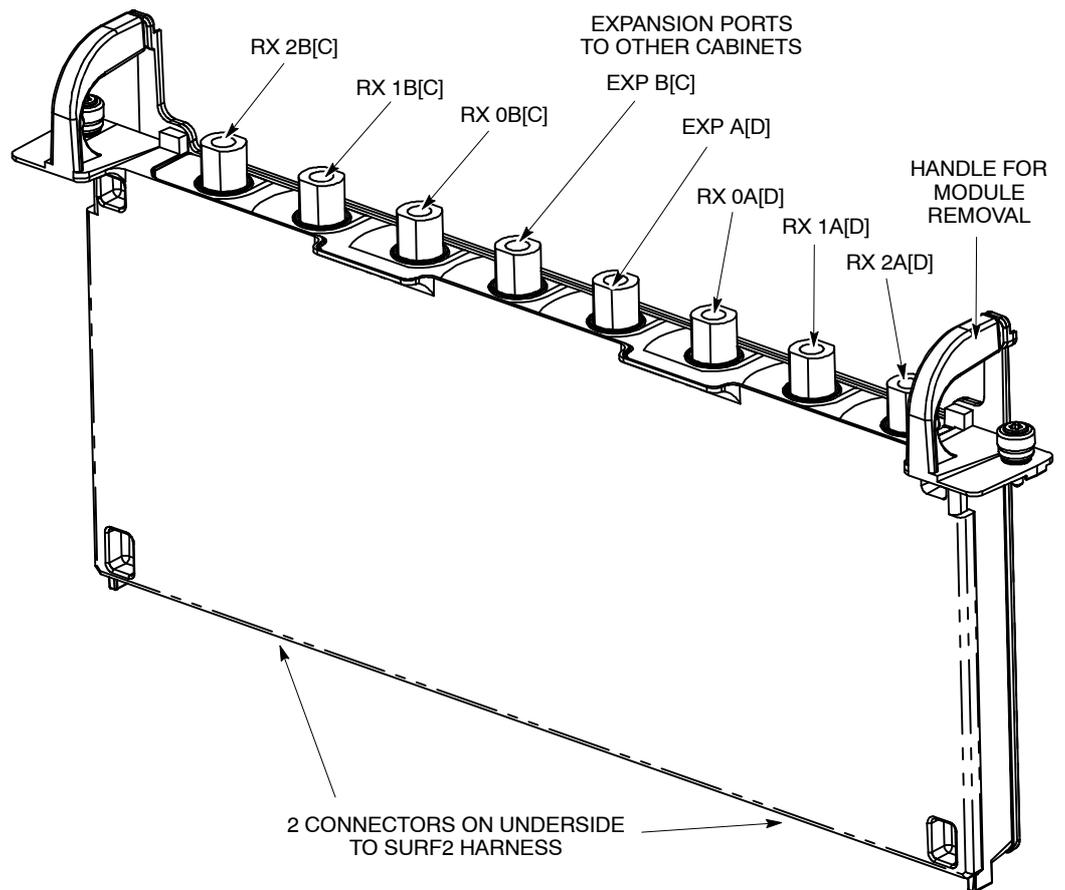
**NOTE** Letters in brackets in Figure Maint. 2-11 refer to the port numbering on the second (optional) SURF2.
