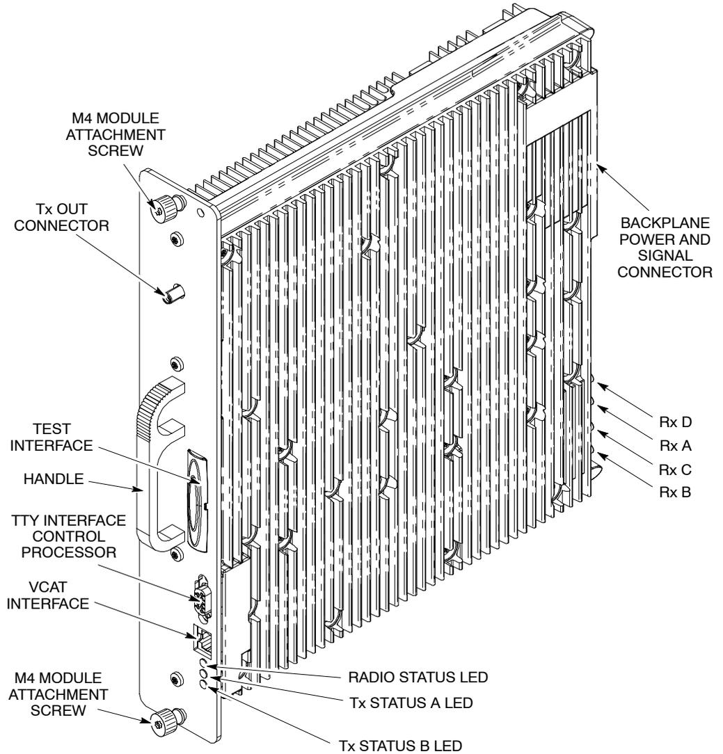
**NOTE** Rx A (main branch) and Rx B (diversity branch) are the only Rx connectors used in a cabinet containing a single SURF2. Rx C (branch 3) and Rx D (branch 4) are only used when a second SURF2 is installed in the cabinet to provide four branch Rx diversity.
