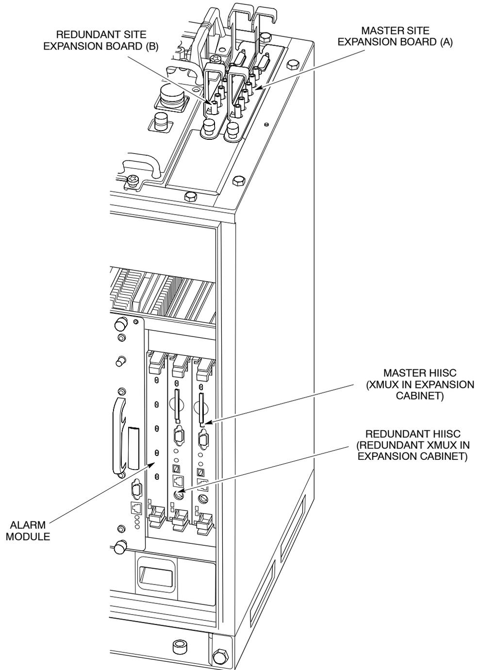
**NOTE** Site expansion boards are only required when expansion cabinets are used.
