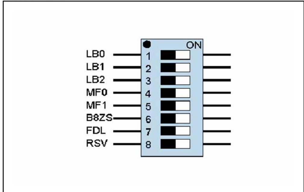
The E1 or T1 mode selection is performed through to switch SW10. Refer to the following tables for detailed information on E1/T1 configurations of the ICM Abis switches.
