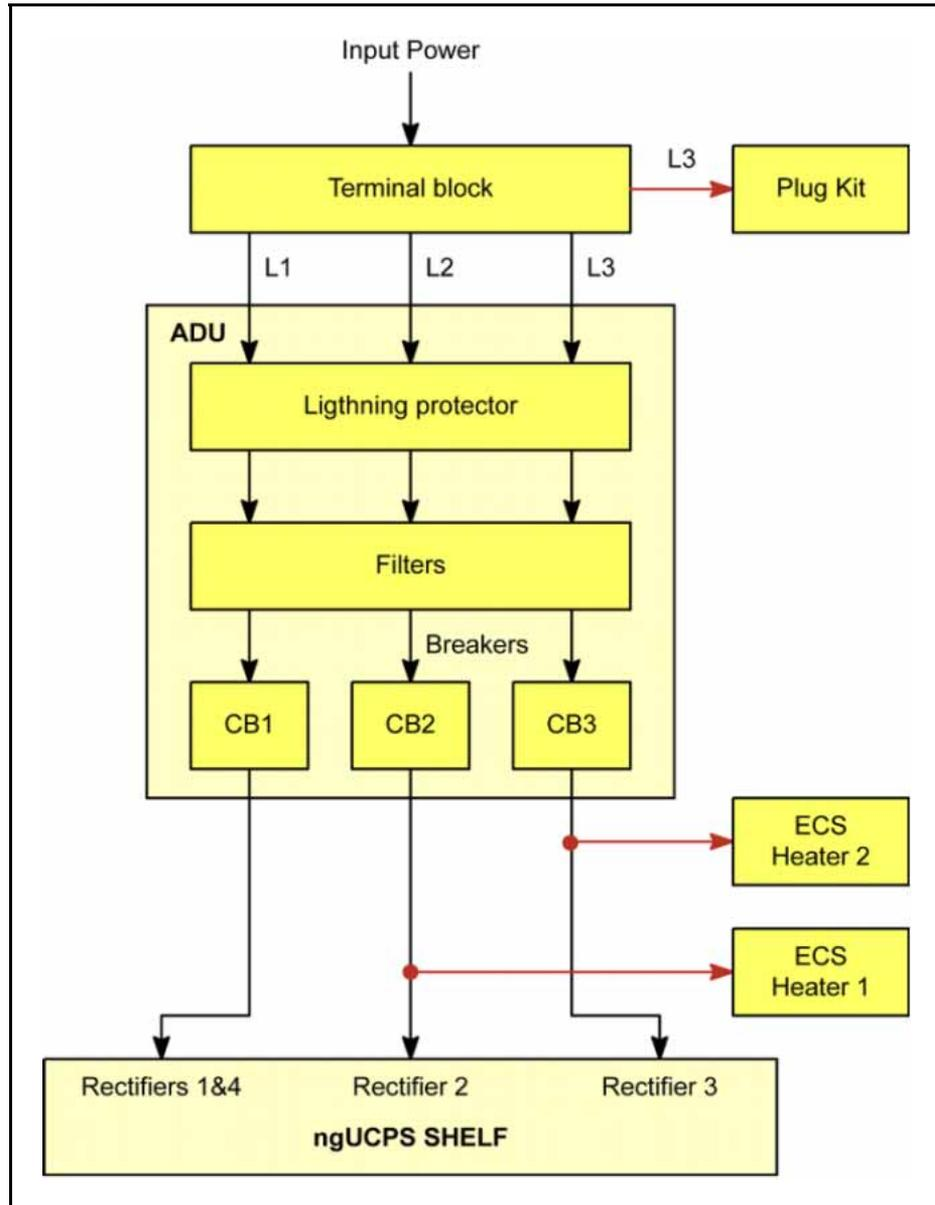
**AC plug types** The optional AC plug kit enables user devices to be plugged during the installation phase. A differential circuit breaker protects the service personnel against injury.
