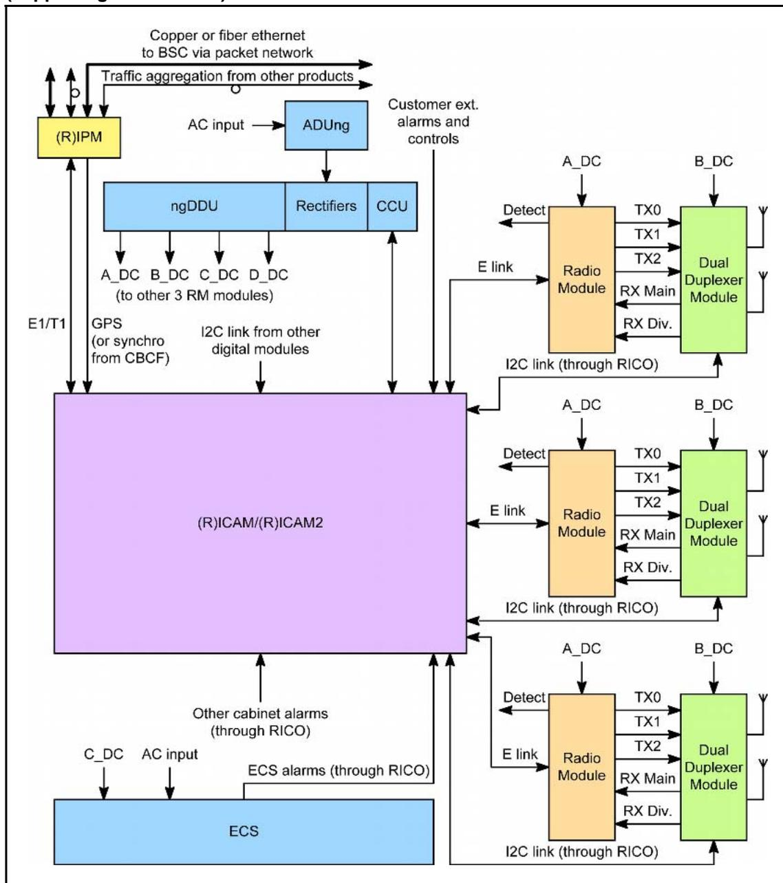
Most of the interfaces between IFM, ICM, ABM and the Radio Modules, as well as primary DC (-48 V) distribution, are performed through the back-planes (IBP/CIBP or DBP).
