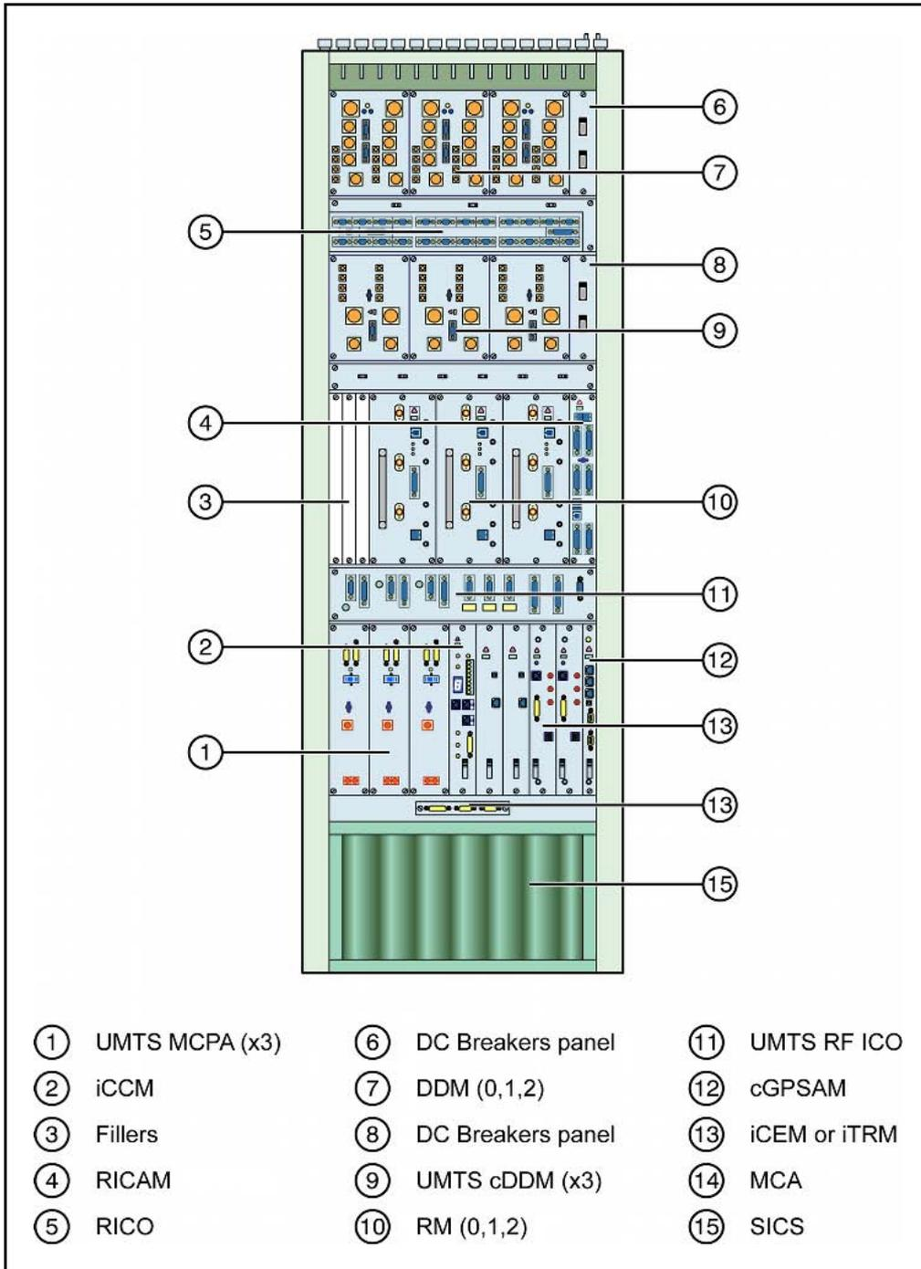
**BTS 18020 - GSM-UMTS (Outdoor combo)** The following figure presents an example of a BTS 18020 - GSM-UMTS cabinet layout and situates the modules in a fully equipped cabinet. This is a configuration with RICAM or ICAM.
