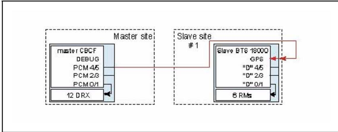
A specific cable is needed between the master and slave BTSs. This cable is a derivation of the PCM between base and extension cabinets of the master BTS that is connected to the GPS connector of the slave BTS 18000 base cabinet.
