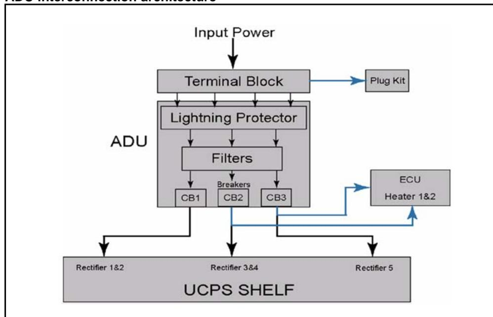
**AC plug types** The optional AC plug kit enables user devices to be plugged during the installation phase. A differential circuit breaker protects the service personnel against injury.
