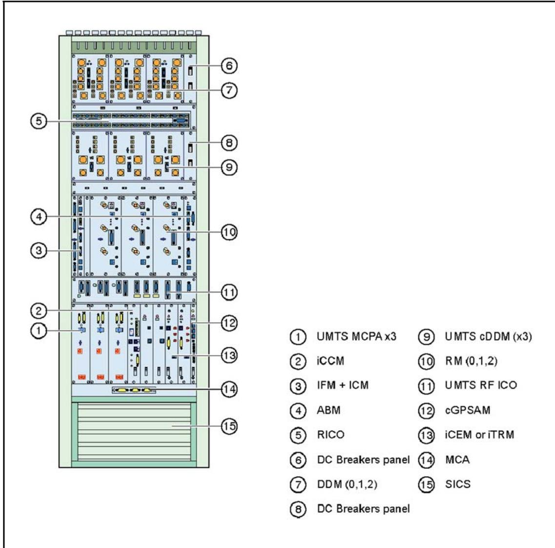
The following figure presents an example of a BTS 18020 - GSM-UMTS cabinet layout and situates the modules in a fully equipped cabinet. This is a configuration with BCF on IBP/CIBP (without RICAM or ICAM).
