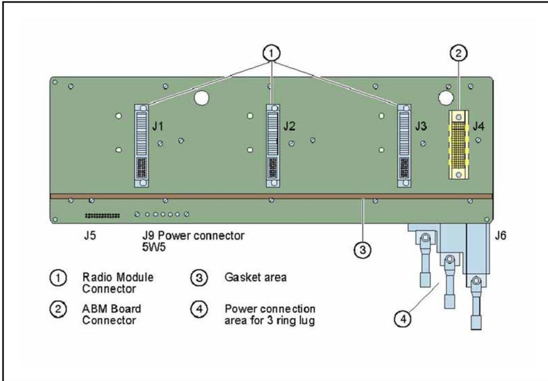
In the preceding figure, the bus bars are shown at the bottom right hand corner (they are indicated as item four).
