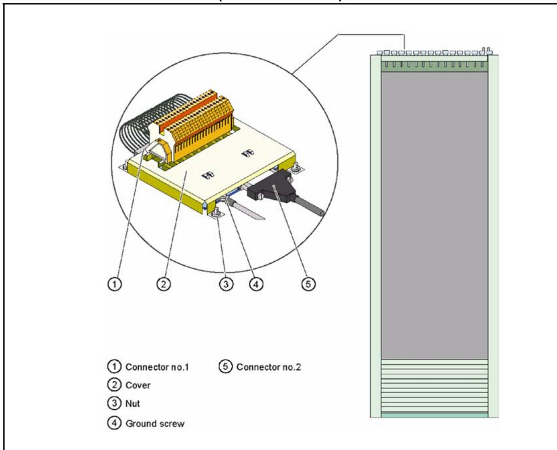
Inside the BTS 18020 cabinet, secondary protection is provided by the ALPRO2 module (see the preceding figure for the location of ALPRO2 module inside the BTS 18020 cabinet).
