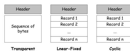
A linear fixed EF consists of a sequence of records of a same length. Data are accessed by record number instead of byte address. Record length and total number of records in a file are indicated in the header.
