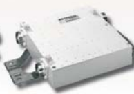
Dual-band Combiner 1710-1880 MHz/ 1920-2170 MHz
