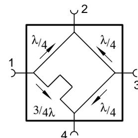
**Note:** VSWR and attenuation are measured when the remaining ports are terminated with 50-Ω loads.
