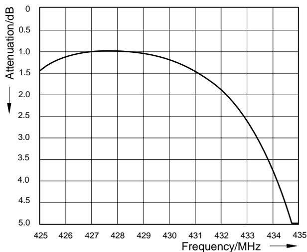
Diagram III: (High band → Antenna)
