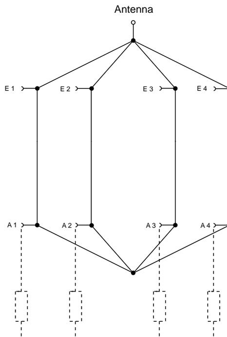
Connectors E 1 ... E 4: Inputs, decoupled
