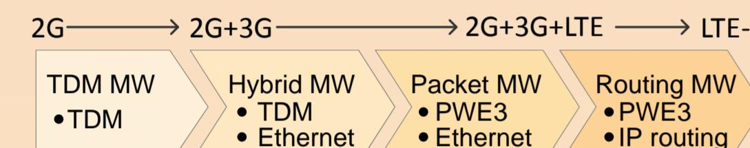
Hybrid/packet/router integrated microwave equipment supports the receiving and encapsulation of multiple types of services, and provides a big pipe for service backhaul.
