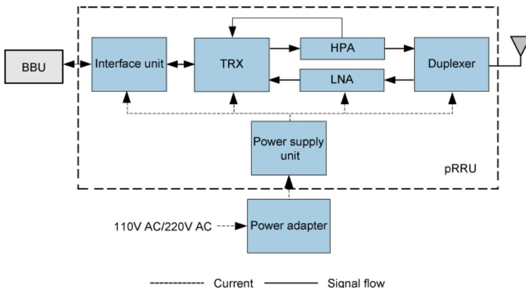
**Figure 3-8** Logical structure of the pRRU3801 with electrical ports
