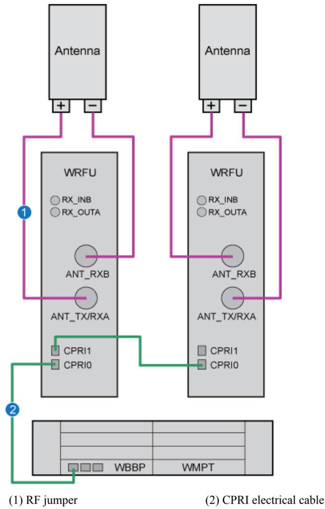
**Figure 4-20** Cable connections of the NodeB in 2T4R configuration (RRU3804 configured)
