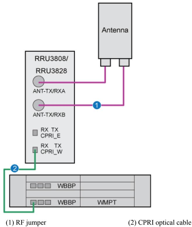
**Figure 4-7** shows the cable connections of the BTS3900C in 1x3 configuration.
