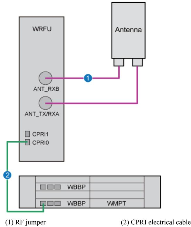
**Figure 4-3** Cable connections of the NodeB in 3x1 configuration (RRU3804 configured)
