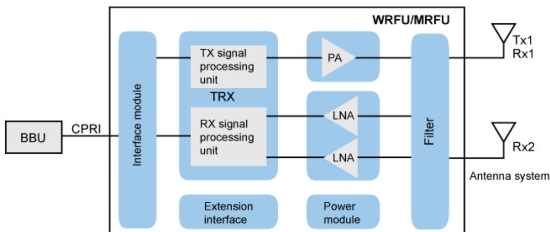
Figure 3-5 shows the logical structure of the WRFUD and MRFUD.
