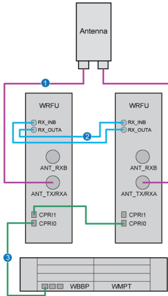
**Figure 4-13** Cable connections of the NodeB supporting transmit diversity (RRU3804 configured)
