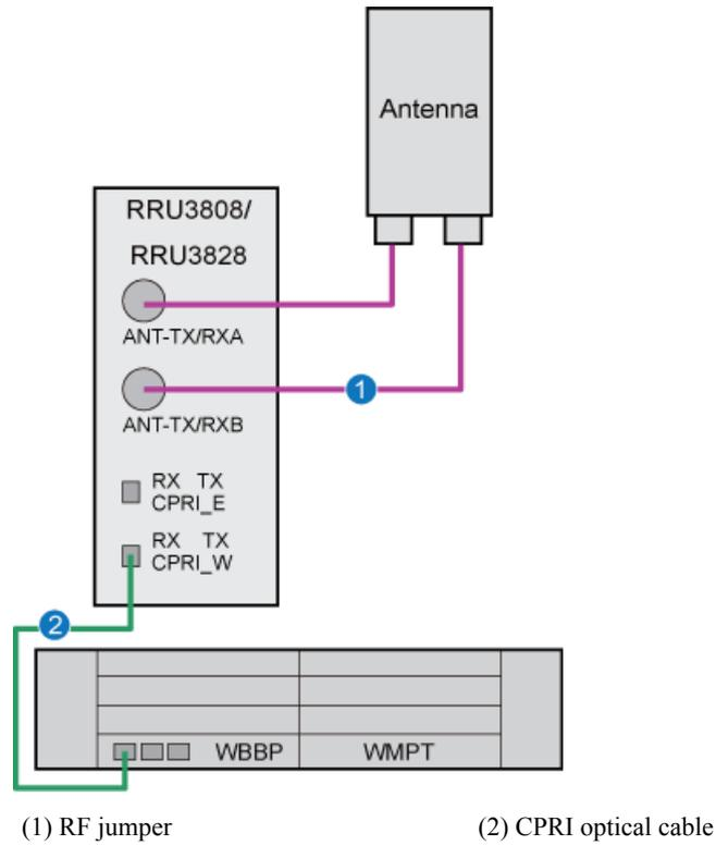
**Figure 4-6** Cable connections of the NodeB in 3x4 configuration (RRU3808, or RRU3828 configured)
