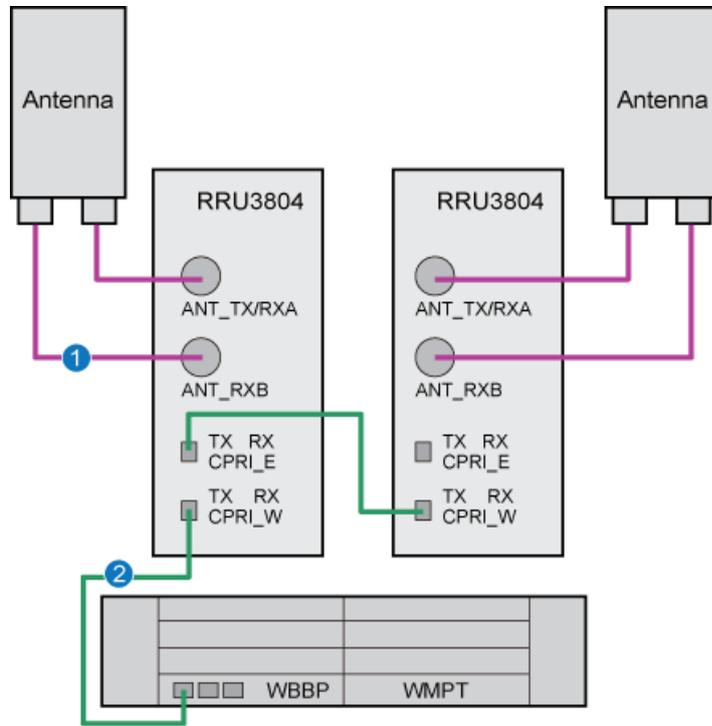
**Figure 4-10** Cable connections of the NodeB supporting 4-way receive diversity (RRU3808, or RRU3828 configured)
