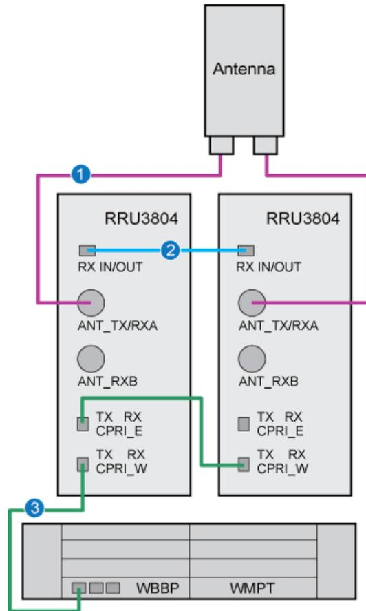
**Figure 4-18** Cable connections of the NodeB supporting 2x2 MIMO (RRU3808, or RRU3828 configured)
