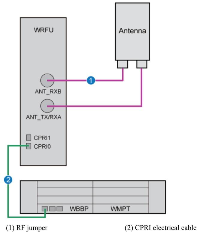
**Figure 4-2** Cable connections of the NodeB in 3x4 configuration (WRFU configured)
