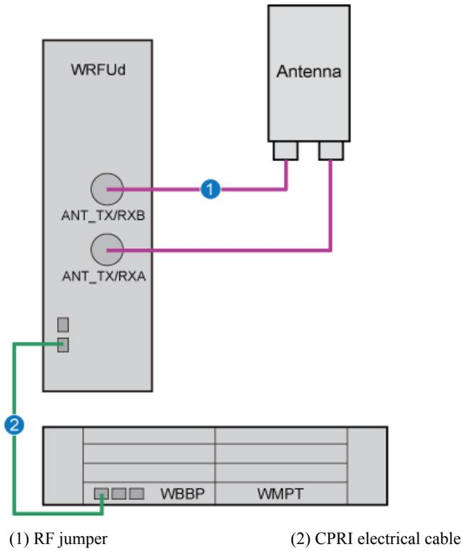
**Figure 4-17** Cable connections of the NodeB in 2x2 MIMO configuration (RRU3804 configured)
