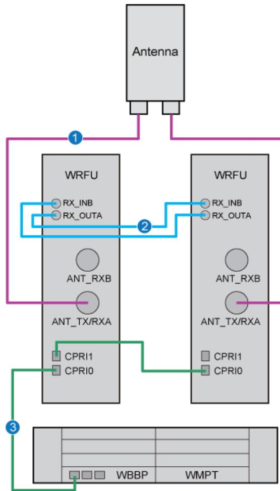
**Figure 4-16** Cable connections of the NodeB supporting 2x2 MIMO (WRFUd configured)
