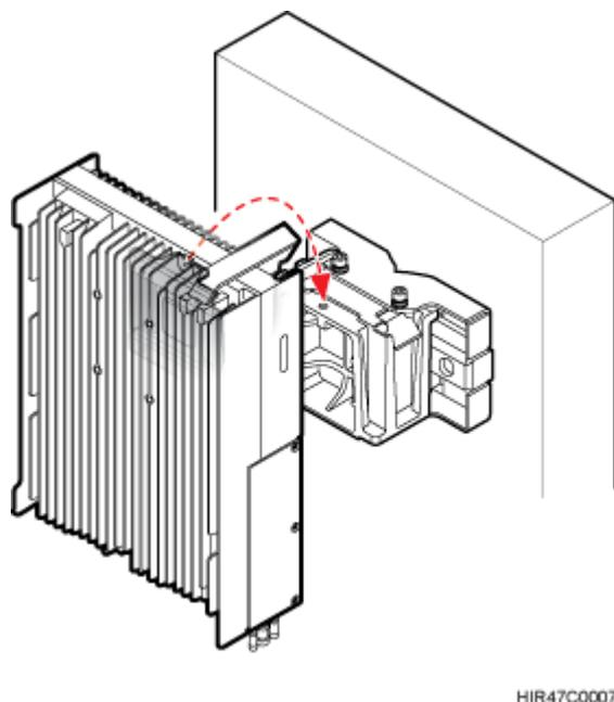
**Step 8** Use an inner hexagon screwdriver to tighten the captive screw into the holes on the top of the attachment plate and main bracket to 5 N·m (44.25 lbf·in.) so that the attachment plate and main bracket are firmly secured, as shown in [Figure 8-41](#).
