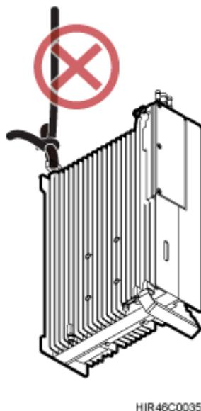
3. Installation engineer B pulls the lifting sling downwards, and installation engineer C pulls the traction sling outwards to protect the RRU from colliding with the tower.
