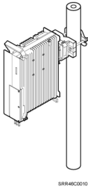
**Figure 3-8** shows two RRUs installed on a pole.
