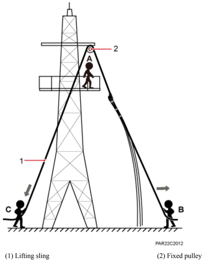
1. After climbing up to the tower, installation engineer A secures the fixed pulley to the tower platform support and leads the lifting sling through the fixed pulley.
