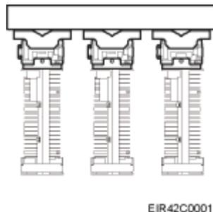
**Figure 3-17** Correct installation of mounting brackets for multiple RRUs installed on an indoor wall in side-mounted mode
