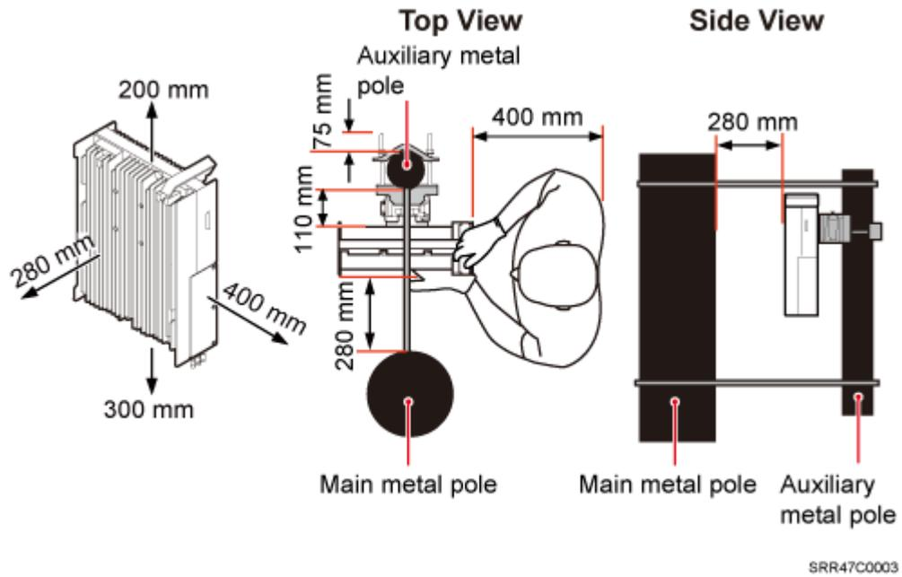
Figure 3-25 Minimum clearance for a single tower-mounted RRU in side-mounted mode
