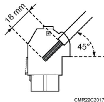
**Step 4** Add a tool-less female connector (pressfit type) to two core wires.
