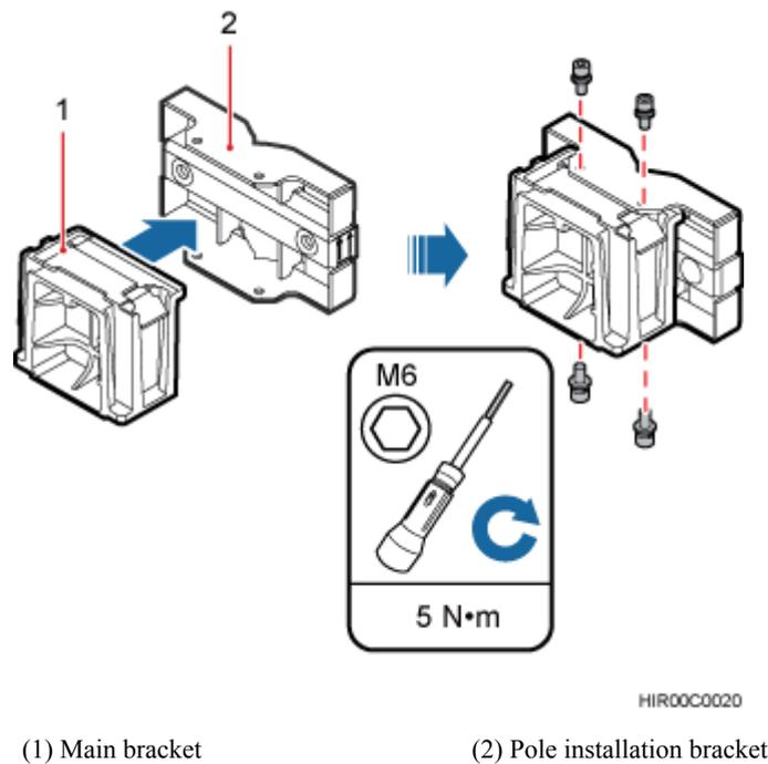
**Step 4** Attach the RRU to the main bracket, and then use an inner hexagon screwdriver to tighten the captive screw into the holes of the attachment plate and main bracket to 5 N·m (44.25 lbf·in.) so that the attachment plate and main bracket are firmly secured, as shown in [Figure 8-46](#).
