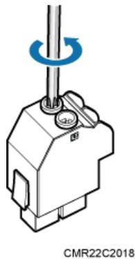
2. Connect the blue core wire labeled NEG(-) to the - port and the black/brown core wire labeled RTN(+) to the + port on the tool-less female connector (pressfit type), and then tighten the screws using a Phillips screwdriver, as shown in **Figure 12-7**.
