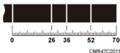
**Step 2** Strip the specified length of the sheath off the power cable, as shown in [Figure 12-3](#).
