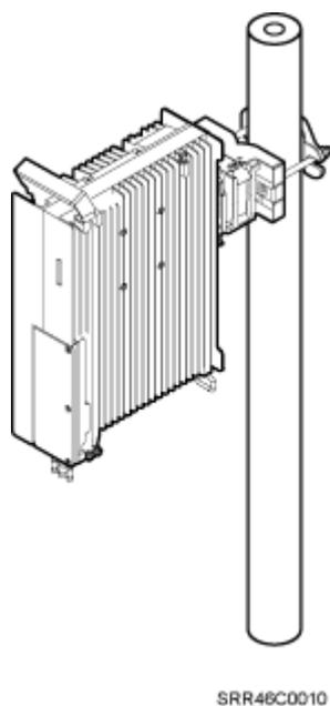
**Step 2** Use an M6 inner hexagon screwdriver to remove the four inner hexagon screws from the second set of mounting brackets, and remove the main bracket from the auxiliary bracket, as shown in [Figure 8-9](#).
