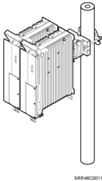
**Figure 3-9**, **Figure 3-10**, and **Figure 3-11** show three or more RRUs installed on a pole.
