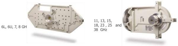
Insertion loss from antenna to ODU is 0,5 dB, return loss 18 dB, Cross-polar discrimination (XPD) 30 dB, Inter-port Isolation (IPI) 35 dB.
