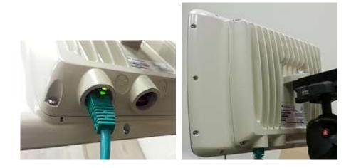
Note: the images above show a LAB radio whose LAN interfaces are without glands. Regular radios are equipped with open gland (LAN port 1) and covered gland (LAN port 2).
