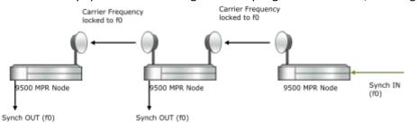
• 9500 MPR has the capability to take any synch input (E1, 2 MHz, 10 MHz, SDH, Synchronous Ethernet, ... ) and to deliver any synch out independently.
