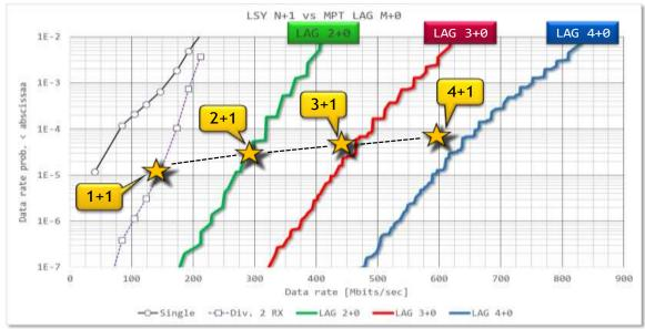
Figure 2 shows a comparison between multichannel in 9500 MPR and performances of the previous legacy ALU platform where protection is based on a traditional N+1 mechanism.
