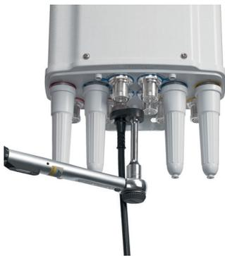
Carefully place the connector and fix the nut using a torque-wrench (according to the manufacturers guidelines).
